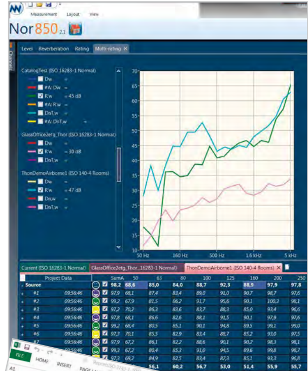
Building Acoustic multi-rating view
