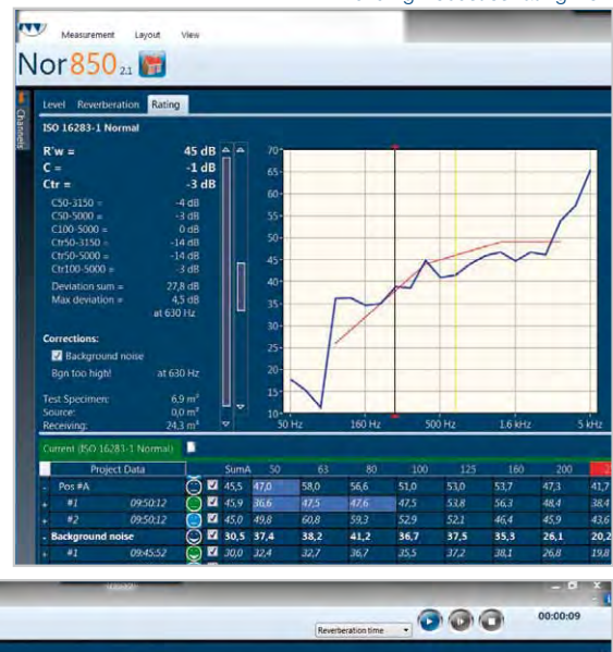
Building Acoustics rating view
