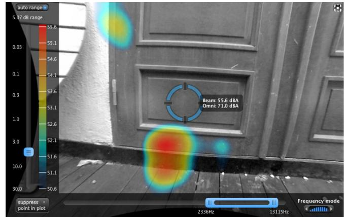
By focusing on the door only it was further possible to locate the exact position of, and zoom in on, those weaknesses as seen in the images below.
