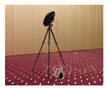
Due to the large size of the modular walls, the camera was pointed to different areas of the walls, and several measurements were made. The individual measurements could then be examined further in post-processing analysis. Due to the source being used at high volume in the sending room, cracks and gaps in the modular walls would appear as small noise sources at specific location on the walls when recording with the acoustic camera in the receiving room.
