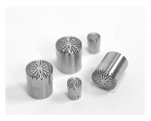
The key components that determines the accuracy of a sound level meter is the measurement microphone and its associated preamplifier. The effectiveness of these components in converting the acoustic signal into an electrical analogue set the maximum accuracy that can be achieved by the ensuing signal processing. Norsonic have a carefully balanced range of measurement microphones to suite a range of applications that complement modern instrumentation yet maintain traditional values.
