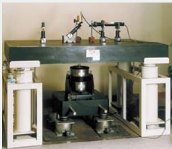
Absolute calibration setup for vibration accelerometers
