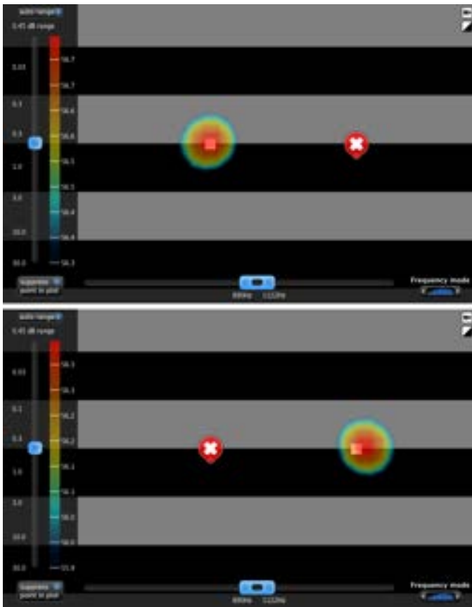
Fig. 15. Using the acoustic eraser to discover two perfectly coherent sources
