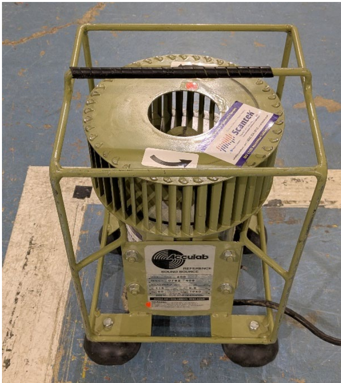
Figure 2 – Detail of sound source
